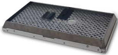
Specimens immersed in temperature controlled water during light or dark conditions rest on mesh insert.
